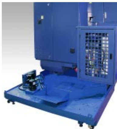
09. Coolant Unit (Chip Rear Disposal)
