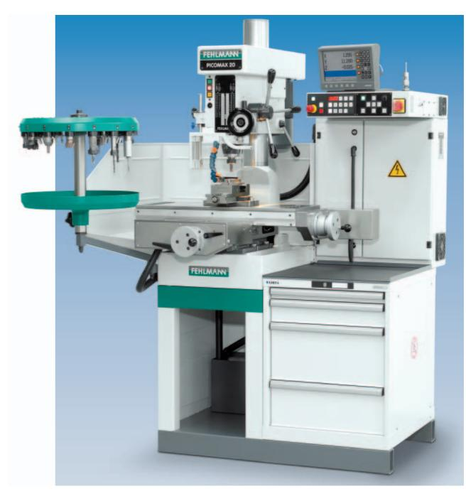
The attached DC motors allow for positioning the table at rapid traverse or by means of the continuously adjustable feed system. All axes of the table are provided with electric limit switches and ball screw spindles. Ideal for milling operations.
