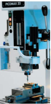
PICOMAX 20 with in-feed system and turret stop with 8 separately adjustable stops for limiting the in-feed.
