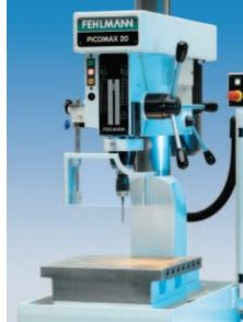
The machine head can be adjusted to different workpiece lengths and heights by means of a crank handle. It is mounted on the column and locked against turning so that the original position on the X/Y axis can be repeated with an accuracy of  $\pm$  0.01 mm.
