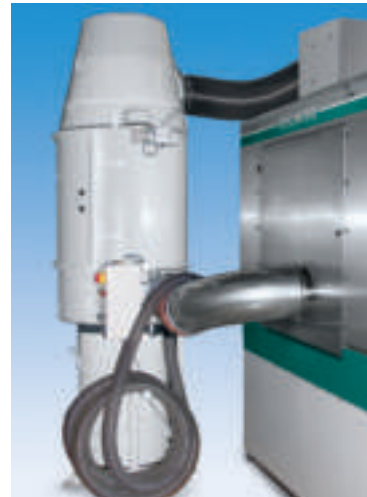
Suction of complete machining area by means of blow and suction procedure.
