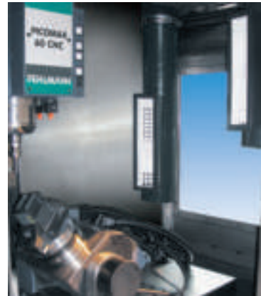
Suction of complete machining area by means of blow and suction procedure.
