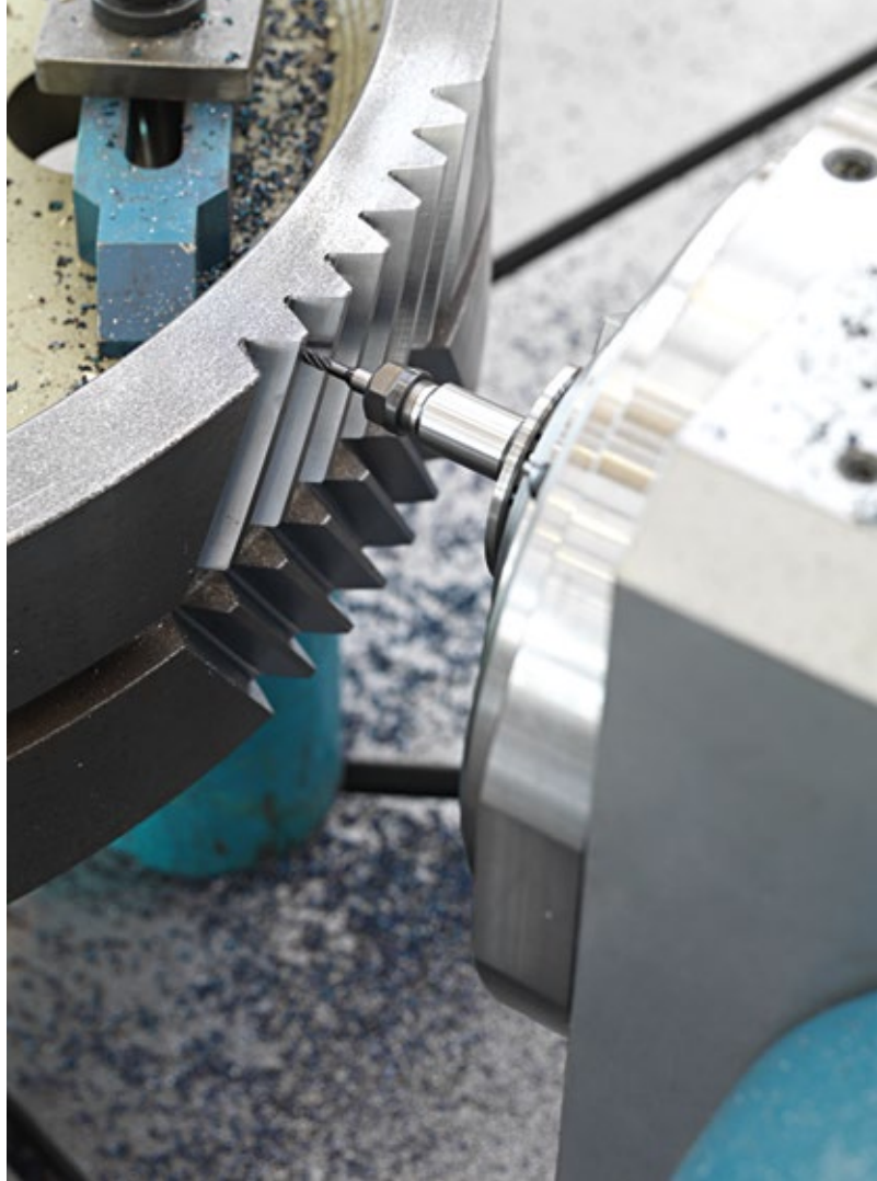
Milling of herringbone gear: tooth profile quality IT7 by milling
