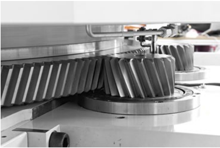
B axis is driven via bull gear and double pinion system (preloaded for backlash free operation)
