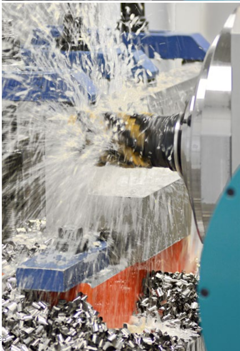
Titanium alloy machining: Ti-6AL-4V material removal rate > 500 cm 3 /min with standard headstock "A" in real production
