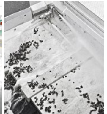
integrated chip washing system
