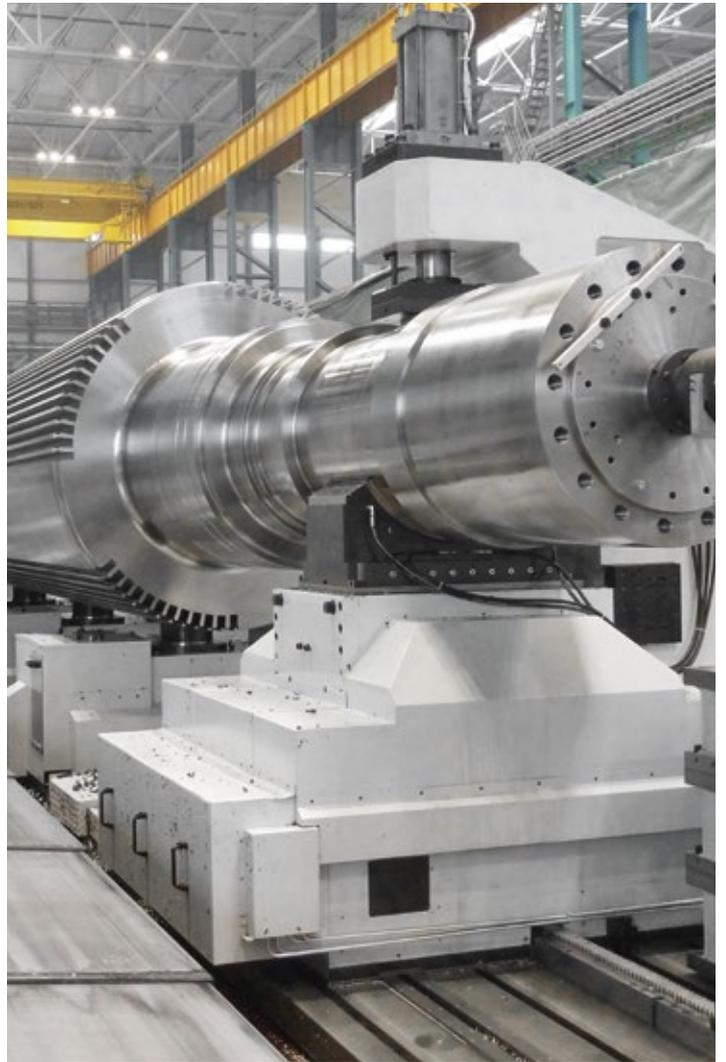
hydrostatic steady rest
