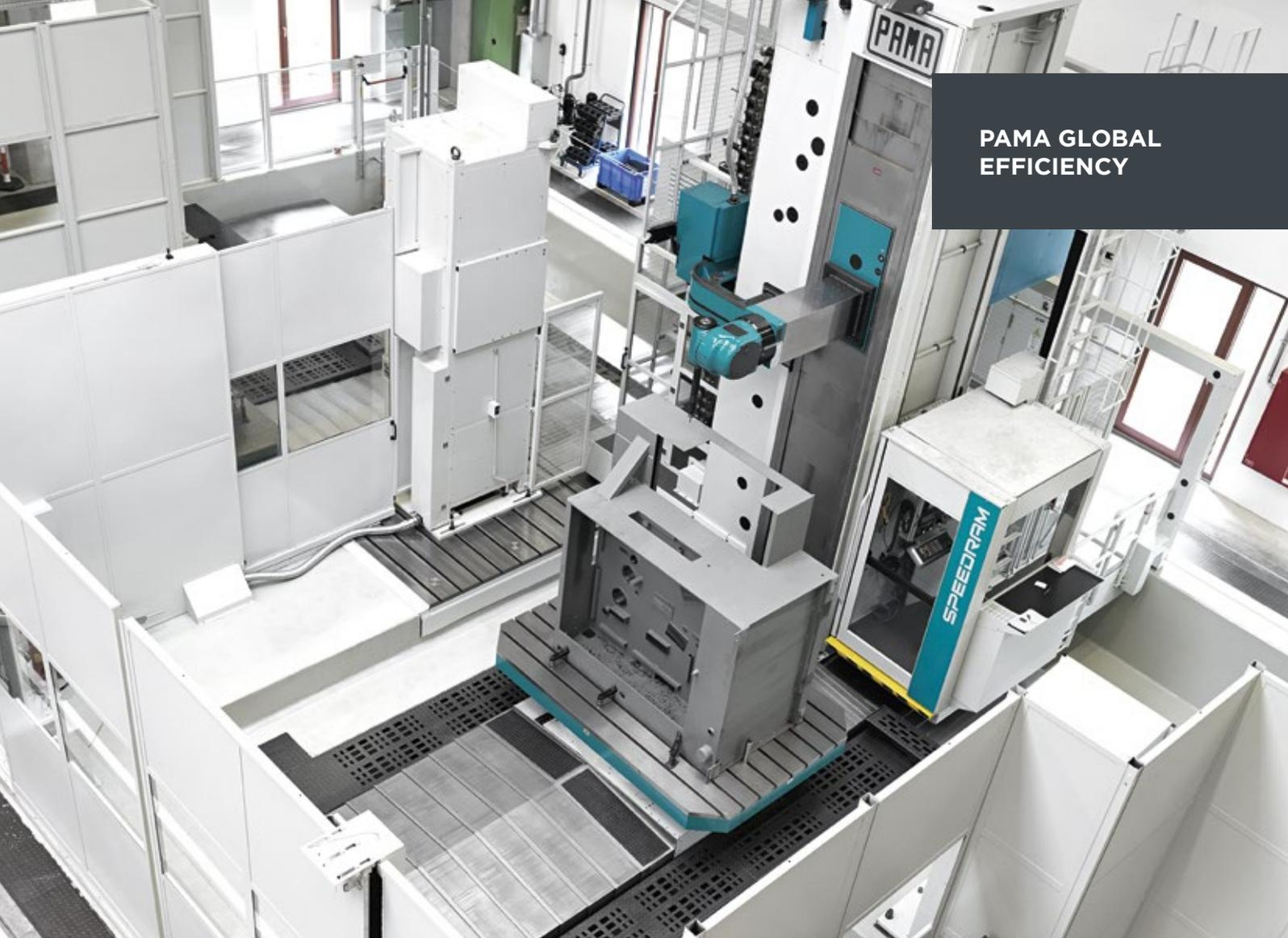
energy saving: low friction guides, use of direct drive technology, regenerating drives, intelligent use of all auxiliary units
