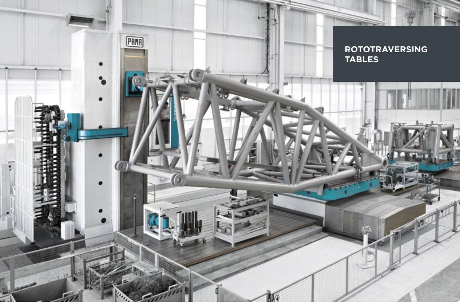
HTC (Hydrostatic Tilting Compensation): automatically detects and compensates the tilting moment created from unbalanced table loads (PAMA patented)
