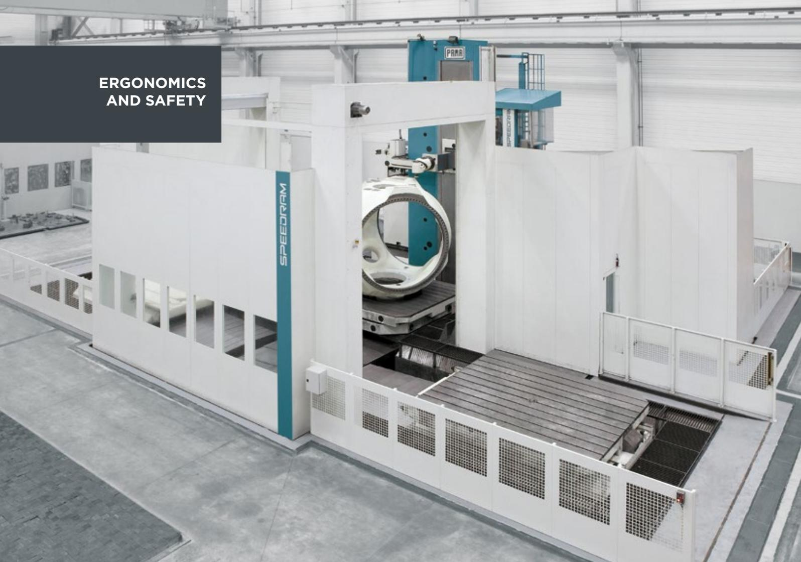
full enclosure systems are available for Speedram machines in order to guarantee a safe and clean working environment
