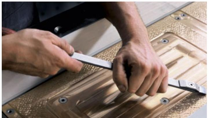
individually hand scraped hydrostatic bronze pads guarantee maximum accuracy of the oil film thickness and performance
