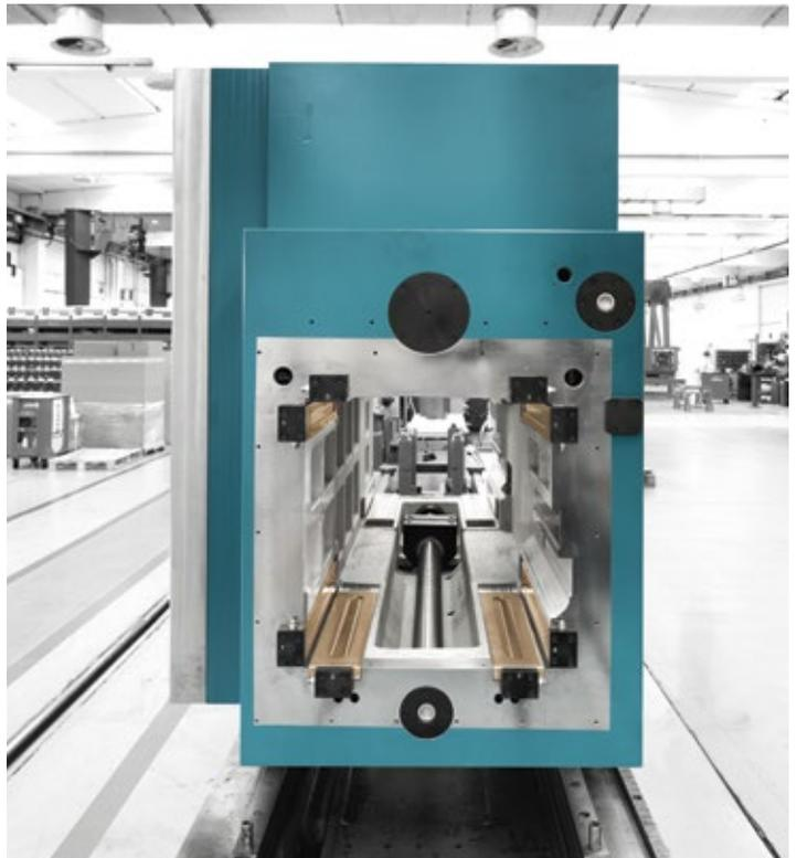
monolithic cast iron headstock with hydrostatic support on all sides
