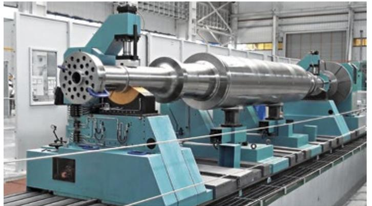
hydrostatic steady rests,
