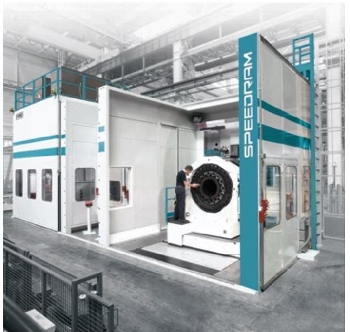
Speedram can be equipped with a large variety of configurations. Multiple table double columns, automatic pallet changing systems or FMS shuttles.
