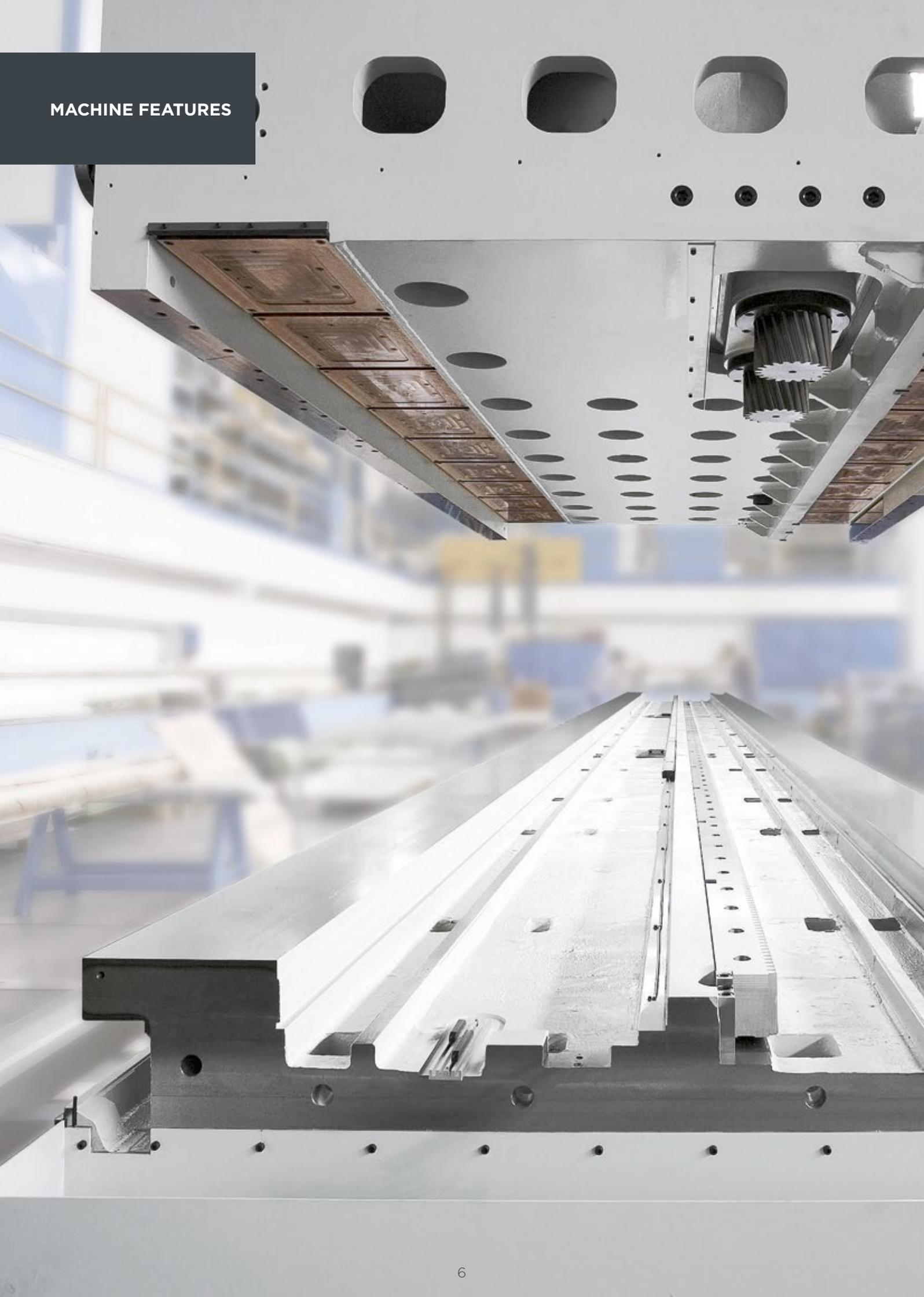
all linear axes with full hydrostatic guideways
