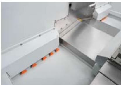
■ Chip flush coolant system increase chips removal efficiency.
