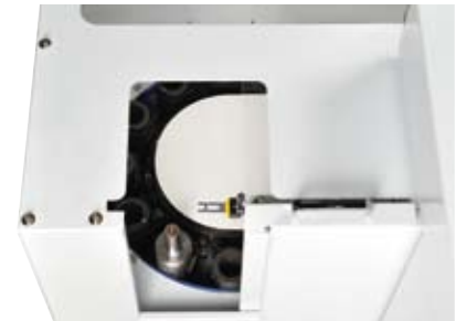
■ Tool magazine with window design is easy for tool changing.
