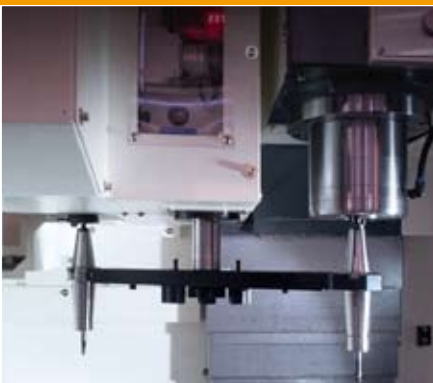
■ Auto Tool Change (T-T): 1.8 sec. IDD PLUS Spindle
