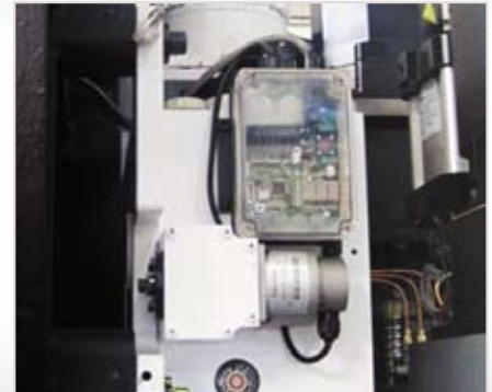
■ Absolute Encoder ATC System < NXV1680B is exclusive >
