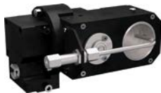
Thread-whirling unit Maximum 5,700 rpm Angle \pm 25^\circ Ø max. 10 mm
