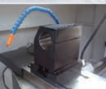
Boring bar attachment mounted on T-slots
