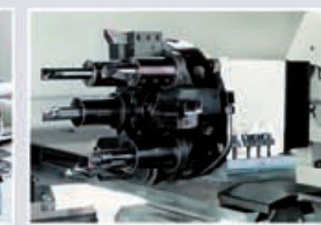
Sauter vertical turret for static tools
