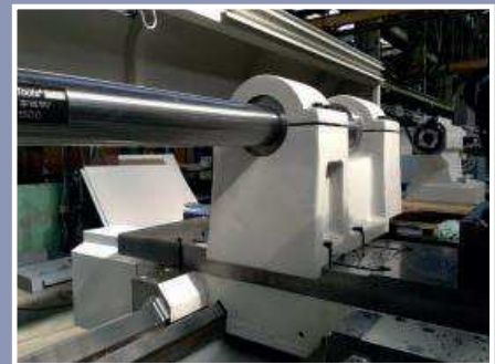
Robust attachment for heavy boring operations
