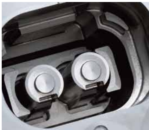
[Connector cavity mold with high aspect features]
