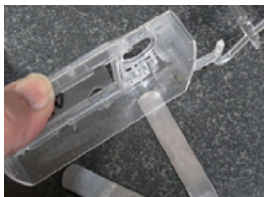
3D cooling water pipe along with product wall
