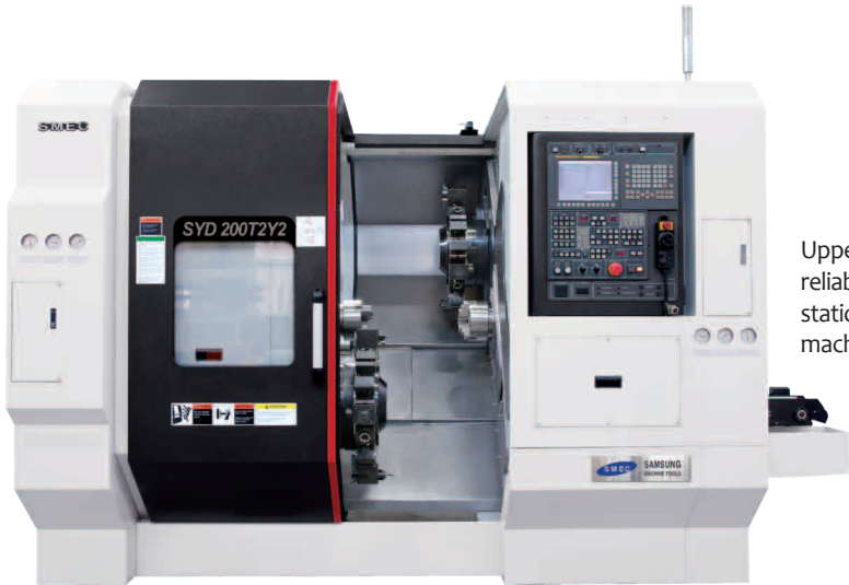
SYD 200T2Y2 Twin Spindle and Turrets for High Productivity
