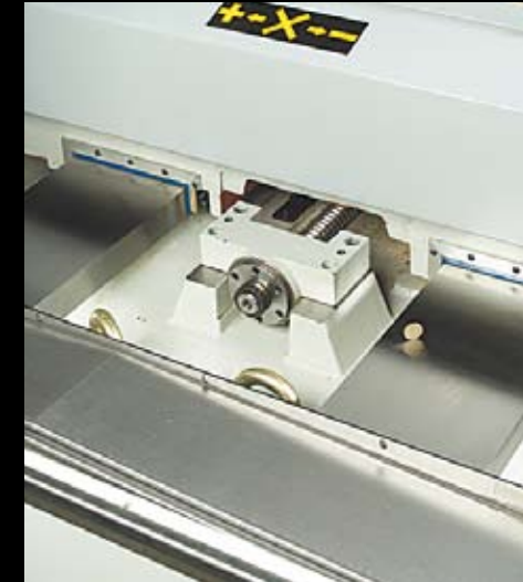
Induction Hardened Box Ways and Turcite coated anti-friction slide ways as featured on: XYZ 560, 710, 1020, 1510, 2010, 2510, and 3010 VMCs.
