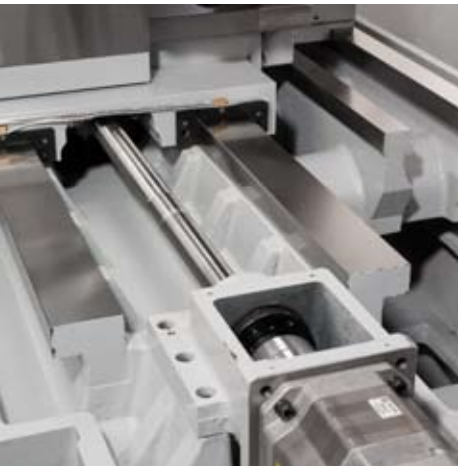
Box Slideways of the XYZ TC 320 LTY The 320 is fitted with large hardened and ground guideways giving superb rigidity and performance.
