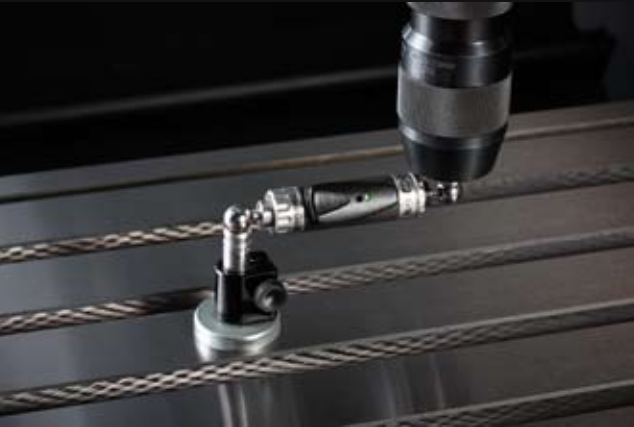
All ProtoTRAK Turret Mills and Bed Mills are Renishaw ball bar tested to ensure accuracy.
