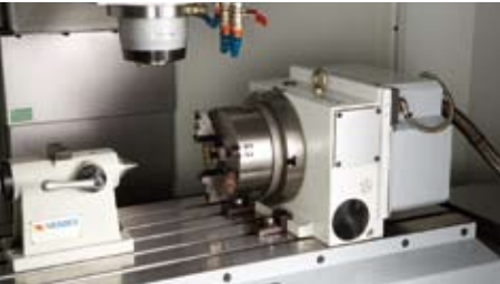
4th axis set up as shown on the 1020.
