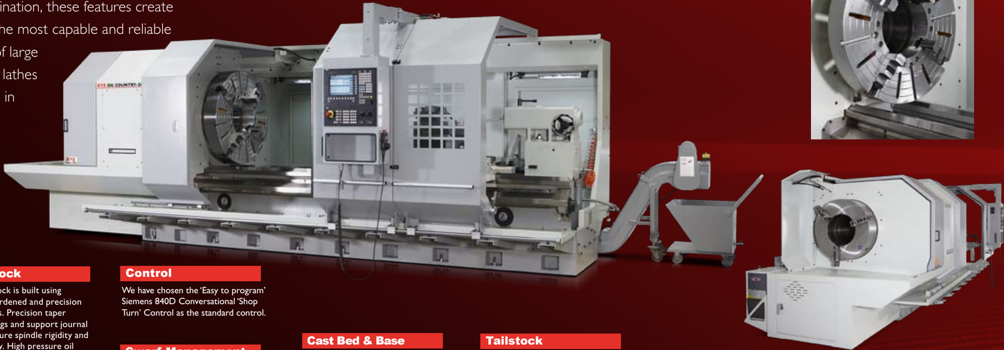
The XYZ Oil Country and XL Lathe range feature a one-piece bed and base casting.
