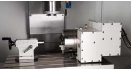
4th axis set up as shown on the 560.
