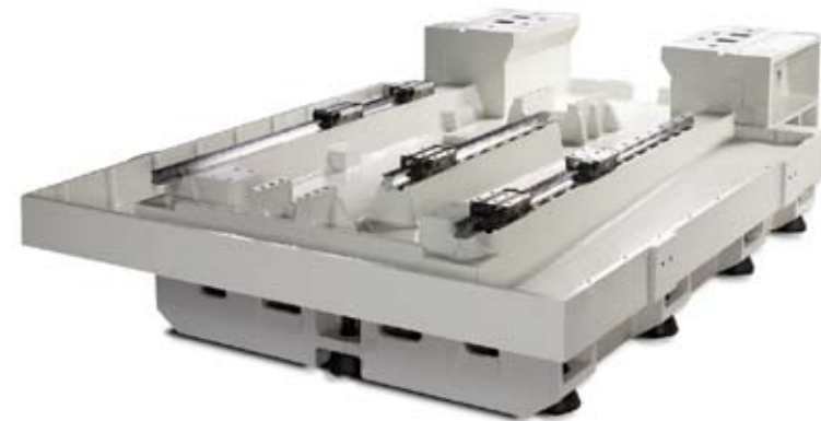
Solid casting showing the three Y axis linear bearings that form the base of this solid cast, rigid, high speed machine tool.
