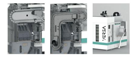
In the basic version, the tool changer with chain magazine offers space for 50 tools (optionally max. 86 tools).
