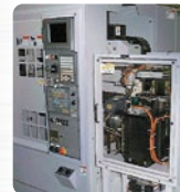
External measurement instrument Dimensional errors are fed back to the machine to maintain high dimensional accuracy.
