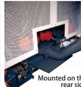
Chip conveyor (Spiral type) Chip disposal is done semi-automatically in the minimum space.
