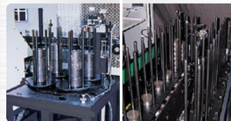
Station stocker Flexible Multi-layer stocker to accommodate different part diameter sizes.
