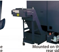
Chip conveyor (Floor type) Chips are reliably discharged outside the machine.
