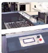
Tray changer Workpieces can be stored together with the tray.
