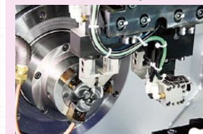
Parallel Hand XW-30, XW-30 PLUS (Σi W30: 2-Axes Control)
