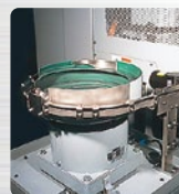
Parts feeder A cylindrical stocker with minimum footprint for storing small parts.
