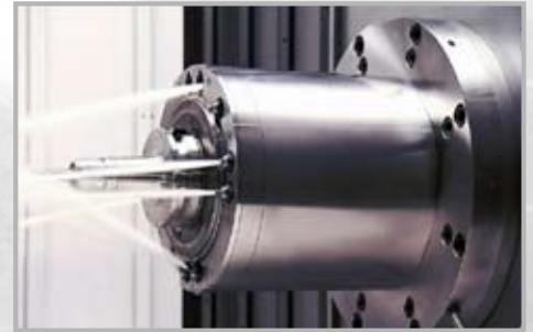
■ 8 spindle coolant nozzles with spindle air blast
