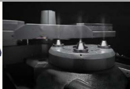
■ Discharging air jet pallet indexing system
