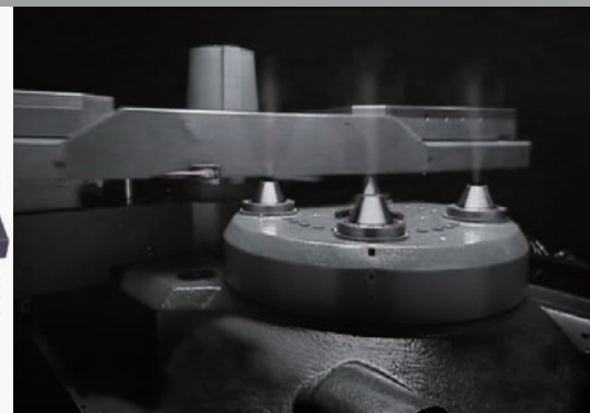
■ Discharging air jet pallet indexing system
