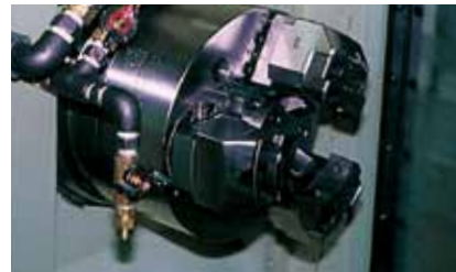
Example of two-way jaws for 6-inch chuck Example of 8-inch specifications
