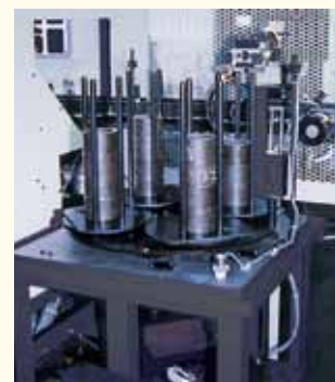
● Rotary Stocker The space-saving, low-cost stocker. The position can be adjusted easily according to the size of the part.
