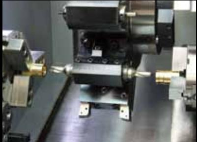
Simultaneous front and back face cutting is available by using the sub-spindle axis.
