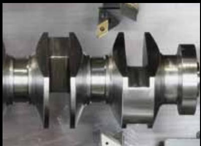
Turrets #1 and #2 are synchronized during OD turning for high precision balance cutting.
