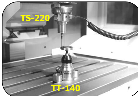
MEASURING DEVICES TS-220: Touchprobe for workpiece measurements. TT-140: Probe for tool measuring.
