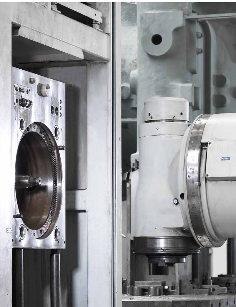
Pick-up station for the automatic exchange of optional accessories
