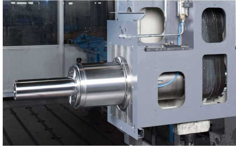
Protruding main bearing of the boring spindle
