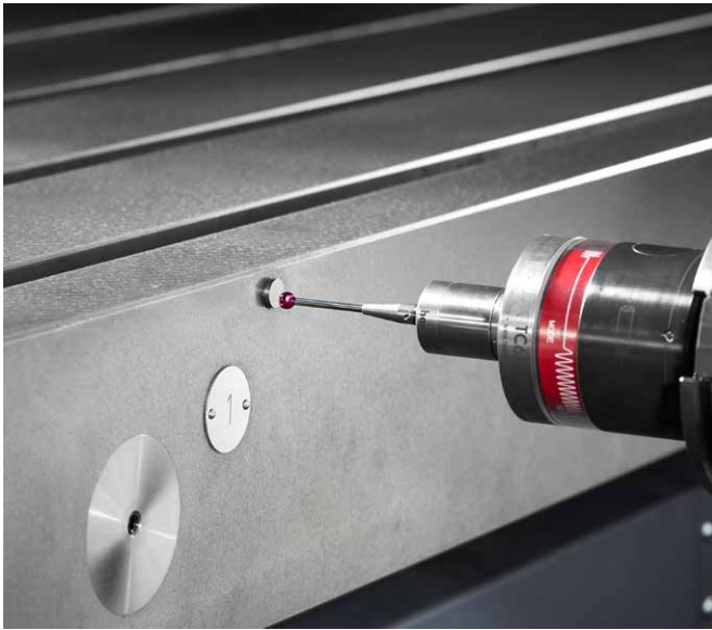
Measuring probe for automatically finding the zero point
