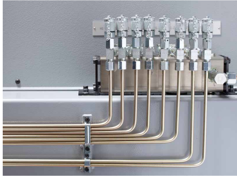
Regulator to regulate the consistent and precise gap distance in the hydrostatic pockets
