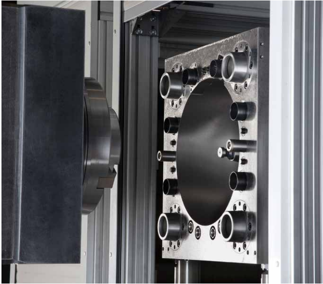
Automatic pick-up of aggregates
