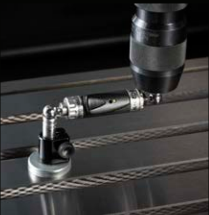
All ProtoTRAK Turret Mills and Bed Mills are Renishaw ball bar tested to ensure accuracy.
