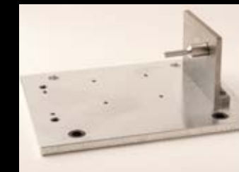
Fixture plate set up - Includes liners, fence, and vice stop assembly.
